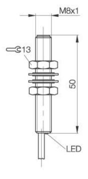
Inductive Sensors BES M08MI-PSC20B-BV02 M 8 x 50 normally-open Sn=2mm shielded
